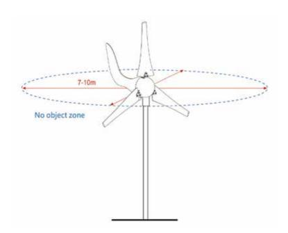
2. The height of installation should be 22 ft (7 m) to 33 ft (10 m). The wind speed below 22 ft (7 m) constrained by the terrain is low and chaotic. For example: If winds in your area are more than 30 mph (13 m/s), a height of 7 m is recommended. The higher the wind turbine stands (more than 10 m), the more stress your pole kit will sustain. Also, the wind turbine possibly brakes in extreme weather conditions.
