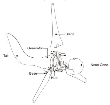
Step 2: Carefully observe windmill layer for easy and quick installation.
